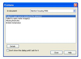
By default, if any warnings or errors of this type are detected when you open a document, the Problems dialog box opens after the document has loaded. You can tell MicroGDS to not automatically open the dialog box by selecting the 'Don't show this dialog until I ask for it' check box.
